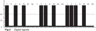
Each degree in the example of a heat detector given the previous section can be expressed in digital form (ie, binary arithmetic). '30' degrees Celsius would then be '11110' and this is what Apollo detectors would transmit. Apollo fire detectors have always used a digital protocol which has remained basically unchanged since its inception in 1986. It has been extended—in two steps, once for XP95 and a second time for Discovery—but never modified.
